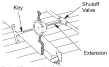
Typical Exterior Wall Gas Shutoff Installation
